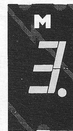
MAN 84 Common Cathode; Right Hand Decimal
