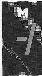
MAN 73 Common Anode; Overflow ( \pm 1 )
