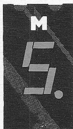
MAN 71 Common Anode; Right Hand Decimal
