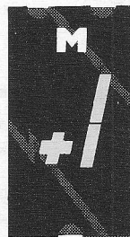
MAN 83 Common Anode; Overflow ( \pm 1 )
