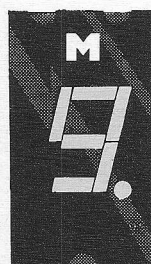
MAN 81 Common Anode; Right Hand Decimal
